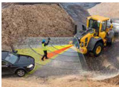
Reversing camera with radar detect
